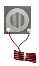
The insulation paste is printed, baked, and hardened on the substate (Fe, Zn, etc.). The hardened insulation layer is then printed with conductive paste (such as Ag), baked, and allowed to firm. The resistance between the two electrodes is measured once the pastes have dried. The plate is employed as sensors if resistance is more than  $16\Omega$ .
