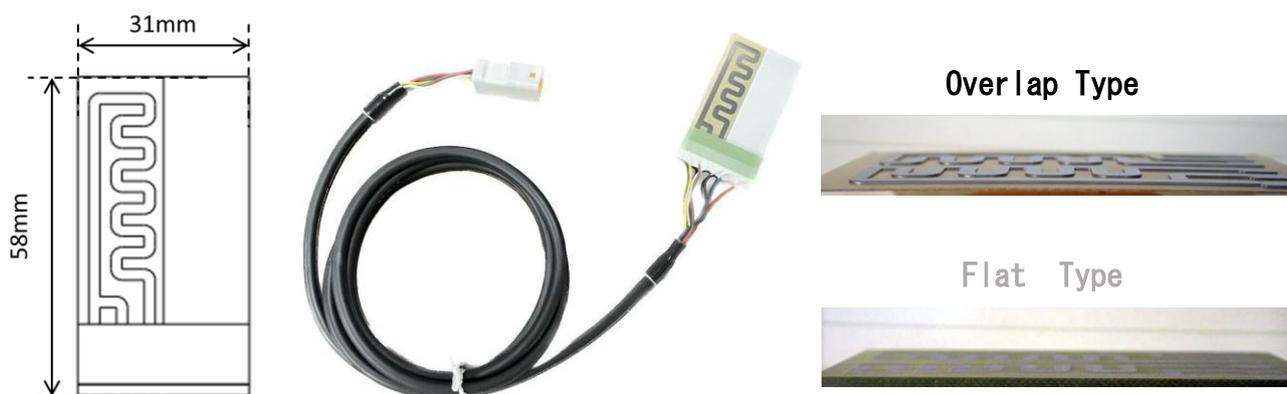
The above figure shows a standard size sensor made of carbon steel. It is possible to change the metal material and electrode shape according to the customer's request. In addition, there is also a type with a thin substrate for installation and measurement in close contact with curved surfaces, and a flat electrode surface for compatibility with plating materials.
